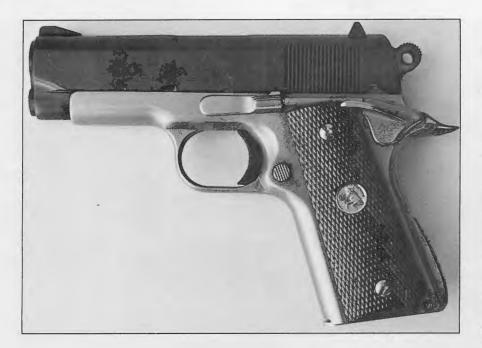
barrel is forced downward and away from the slide. The barrel's rearward travel ceases when it strikes its stop in the frame, while the slide continues backward to complete extraction and ejection of the empty case before rebounding, by means of the recoil spring, to strip and chamber another round from the magazine.
